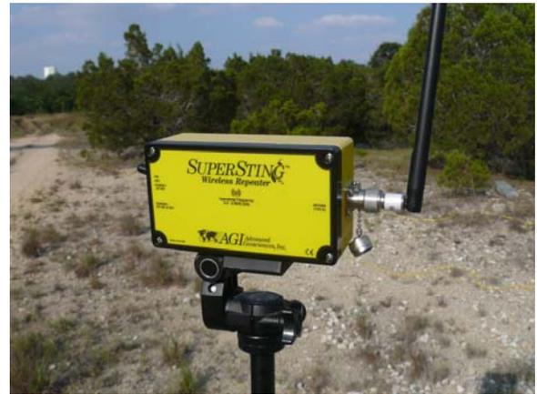
**Figure 24 The SuperSting wireless repeater is placed high on a tripod.**
