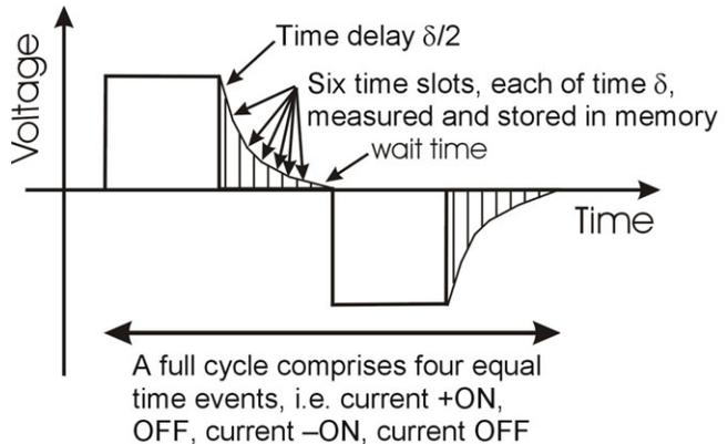
**Figure 36 IP measurement parameters**
