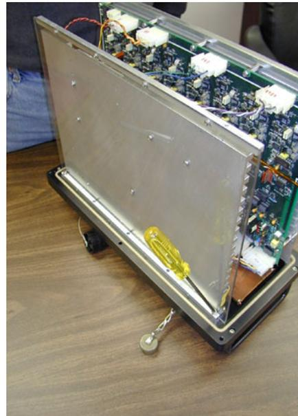
**Figure 46** *Unscrew the five hex screws, holding the transmitter board mounting plate to the front panel.*
