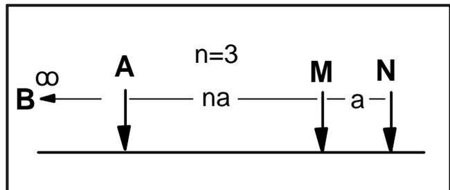
**Figure 12 Pole-dipole electrode array**
