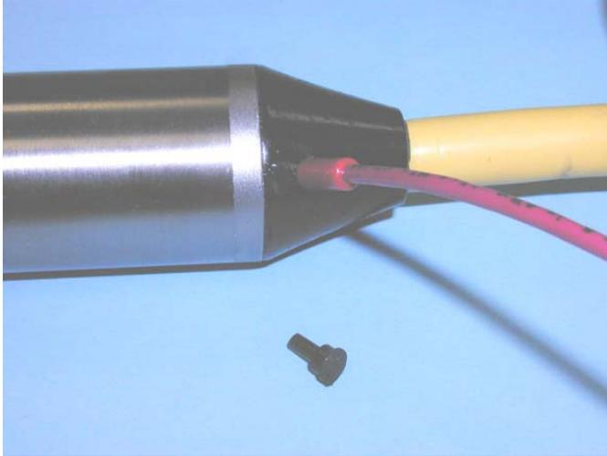
**Figure 40 Remove the plastic plug using your finger nails**
