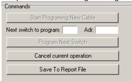
Once this button is pressed the software will begin to scan the serial number of the switch and program the switch with the corresponding address. If this is successful, it will return with a program address successful message.
