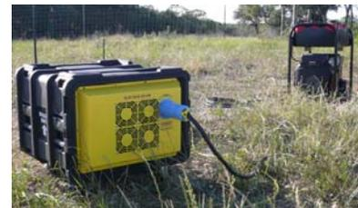
**Figure 23 Caution: blocking ventilation will cause the PowerSting to overheat.**
