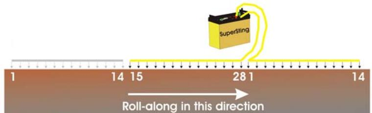
**Figure 6 Data is first collected using cable section 1-14 and 15-28 to the left in the picture. After the initial data is recorded cable section 1-14 is moved to the right and connected to the SuperSting which also has been moved forward**
