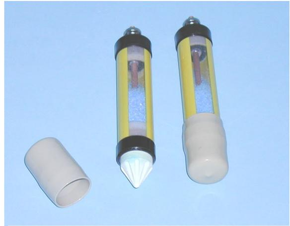
**Figure 44 Non-polarisable electrodes**
