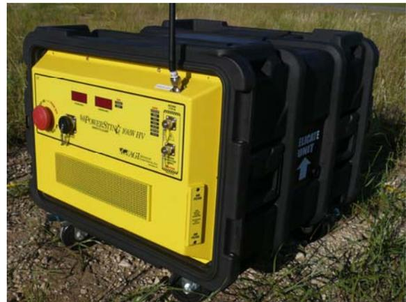
**Figure 22 The PowerSting with the red "kill switch" on the left side.**
