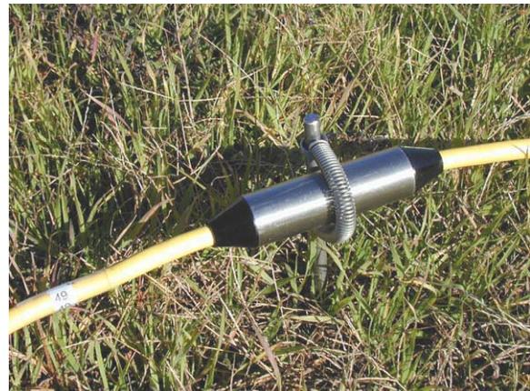
**Figure 2 Attach the electrode switch to the stake by using the stainless steel spring**
