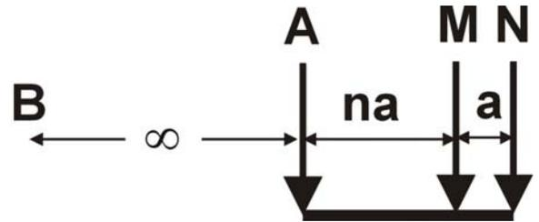
When performing pole-dipole surveys, try to place the B electrode at 10 times the largest expected ( $na+a$ ) distance away from the survey site.
