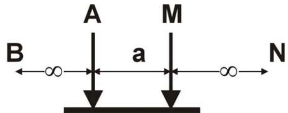
When performing pole-pole surveys, try to place the B and the N electrodes at opposite sides of the survey area and at 10 times the largest expected  $a$  away from the survey site.
