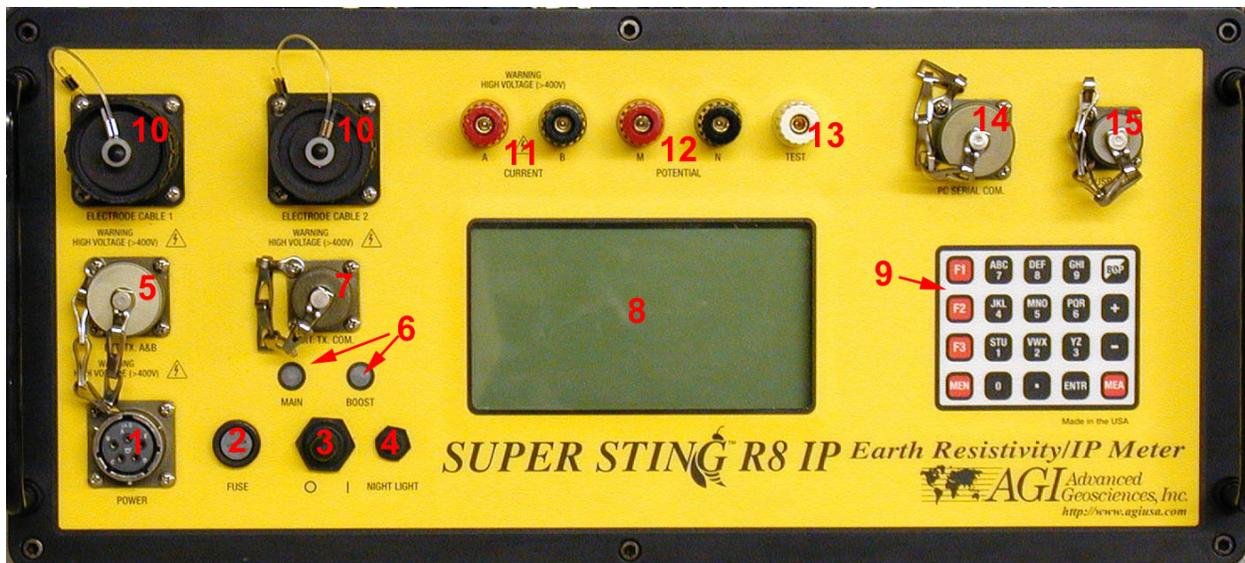
**Figure 8 SuperSting R8/IP front panel**
