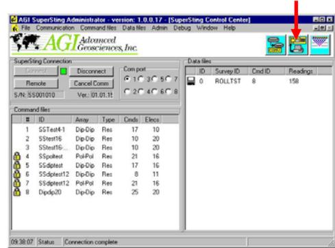
**Figure 17 Use the command center window to upload command files and download data files**
