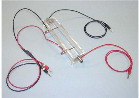
**Figure 34 Test box for soil samples.**
