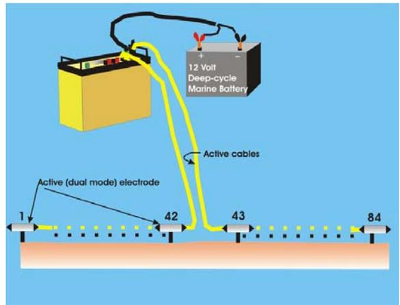
**Figure 3 SuperSting set-up with active (dual mode) electrodes**
