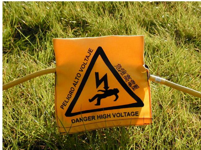
**Figure 1 Use the electrode warning covers**
