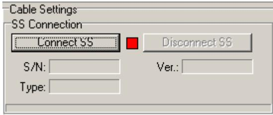
After pressing the “Connect SS” button the PC should connect to the SuperSting and all buttons and windows in the Administrator should become active.
