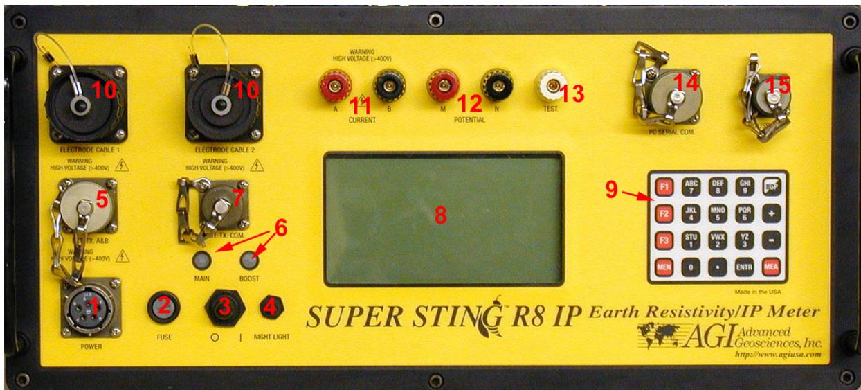
**Figure 8 SuperSting R8/IP front panel**
