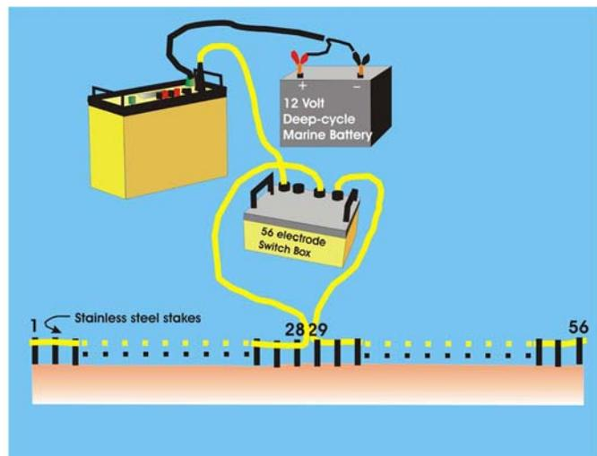
**Figure 27** SuperSting/Switch box connection
