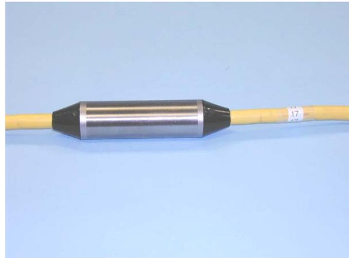
**Figure 42 New style dual mode electrode switch**
