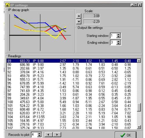
**Figure 21** To speed up inspection, several decay curves can be displayed at the same time
