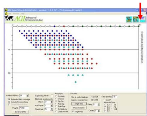
**Figure 16 Use the command creator window to create a command file**
