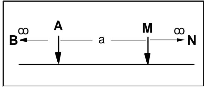
**Figure 13 Pole-pole electrode array**
