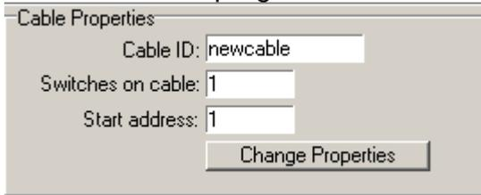
6. In the “Cable Identifier” box enter the serial number of the current cable section. Then in the “No. of Switches” box enter the number of switches on the cable section. Finally enter the Start address of the cable section, which is the lowest electrodes address on the cable section. The following shows the setup for a cable section of 4 electrodes with addresses 5 through 8.
