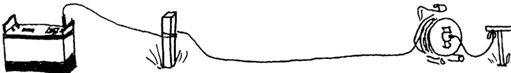
**Figure 28 Tie off cables to some fixed object to prevent cables from accidentally being pulled out of the instrument when the electrodes are moved.**
