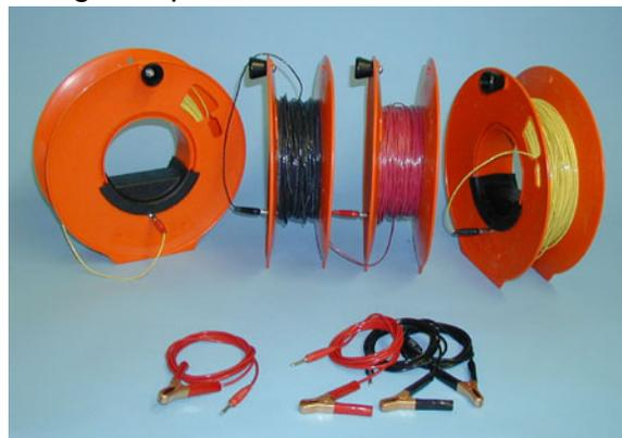
**Figure 20 Short cable set, current 2x150 m, potential 2x50m.**
