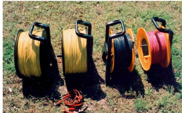
**Figure 22** *Long cable set, current 2x750 m, potential 2x250 m.*
