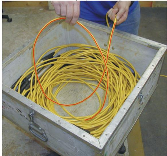
*Figure 5 Incoming cable "under" the loop.*
