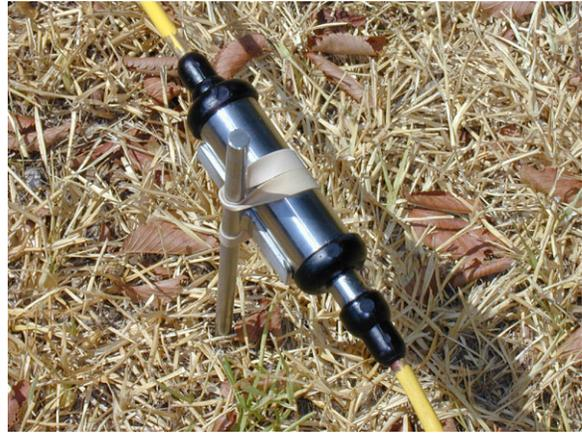
**Figure 6 Rubber band each switch to its electrode stake.**
