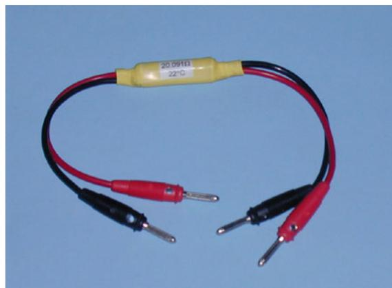
**Figure 33 Test resistor.**
