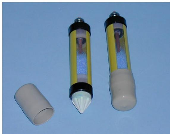
**Figure 25 Non-polarisable electrodes.**
