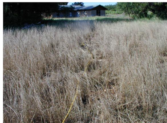
***Figure 23 It is not easy to find the stakes once the cable is gone (left picture). Instead follow the cable and pick up the stakes before picking up the cable (right picture).***
