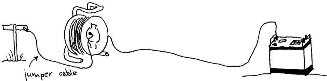
**Figure 27 Place the cable reel close to the electrode, not the instrument. Use a jumper cable to connect the reel to the electrode.**
